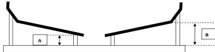
**Dimension A = 195 mm** from the top of the launching trolley axle to the underside of the trolley bunk measured by the inner face of the inner leg.
