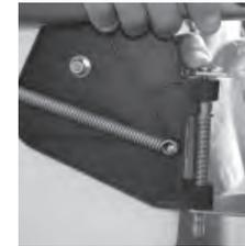
2. Press down on the top of the pintle pin (compressing the pintle spring) and slide the pin's indentations into the gudgeon.
