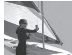
2. You will need to assist the lower boom close to the gooseneck while pulling on the halyard. Continue to pull on the halyard until the upper boom is right against the top of the mast.
