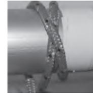
2. Lead the tail of the halyard over the fall (The fall is the remainder of the halyard) and around the upper boom again.
