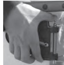
1. Slide the tiller and extension underneath the wire bridle. The pintle pin will have two indentations that align with the two notches in the gudgeon (located on the stern of the boat). Align the pintle pin with the gudgeon notches.
