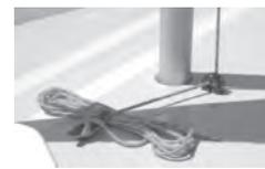
**Tip:** It is suggested to coil up the remaining tail of the halyard and place it under the taught halyard section on the deck. This will keep the halyard from dragging in the water.
