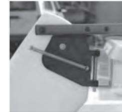
3. Release the pin. The rudder should now be securely attached to the boat. The rudder should be able to pivot from side to side easily. Leave the rudder in the kicked up position prior to launching.
