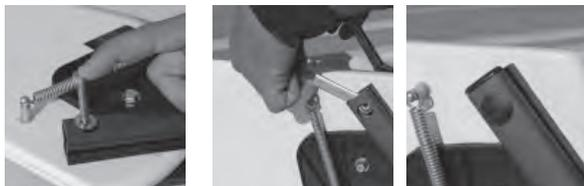
4. Place the plastic end caps on tiller ends and rubber bolt holes.
