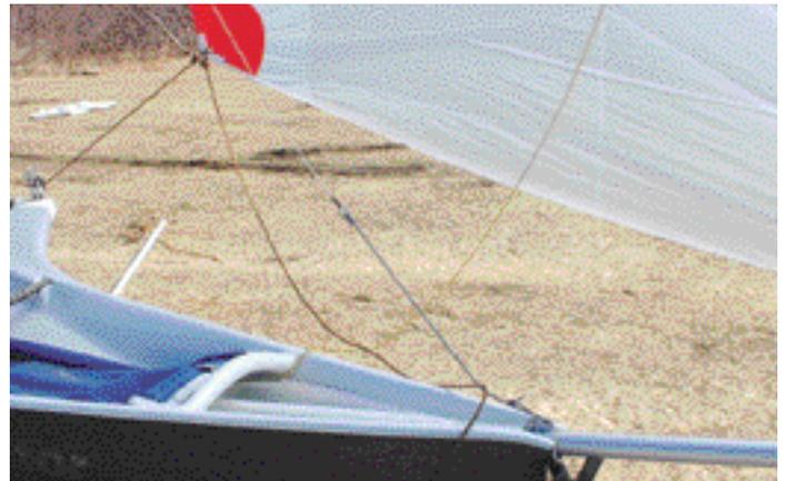
Correctly set up and hoisted spinnaker
